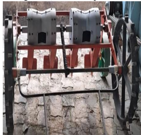
Name of Implement- Rice- Wheat seeder Hiring rate (Without Operator)- 600 Rs /ha
