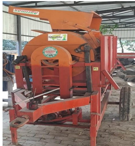
Name of Implement - Multi crop thresher Hiring rate (Without Operator)- 90 Rs /hr
